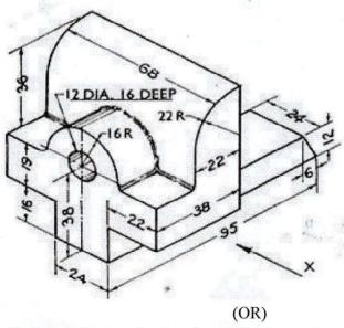
b) Draw the Isometric view for the given following orthographic view. 14(M) CO5 L5
